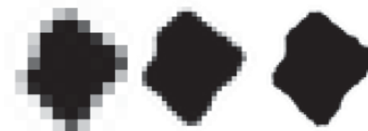
Figure 5: Representation of a grain from Krumbein's 90% class at different densities ranging from 70 to 1750 and 7 000 pixels.
